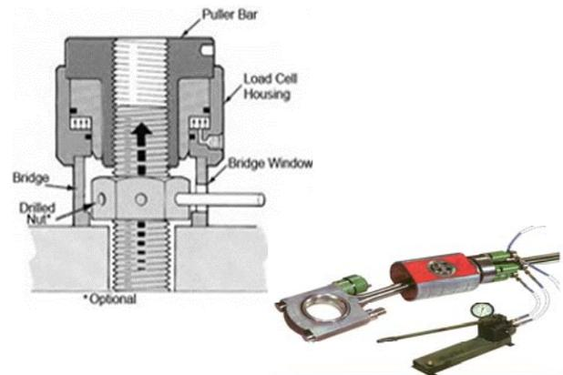
Hydraulic Tensioning provides a very good compromise on accuracy, practicality, and effectiveness. When utilizing Hydraulic Tensioning; there is also the issue of making sure that the threads on the nut and the threads on the stud have a chance to seat due to the relaxation that occurs as the threads in the nut and stud seat with each other i.e. a small amount of plastic deformation / creep occurs.
