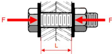
As a fastener creates the compressive clamping force which holds two or more pieces together, there is an equal and opposite force that acts on the faster which places it in tension. This tensile force creates a stress in the fastener. Stress is defined as the applied Force per unit Area. Stress is denoted by the symbol,  $\sigma$ .
