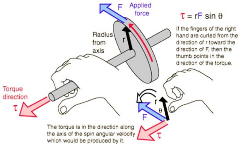
Torque – applied by “calibrated” mechanic arm strength or calibrated torque wrench
