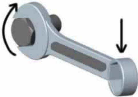
Torque has many variables which make it really only an approximation of bolt stress / force. These variables include the accuracy of the torque wrench and multiple sources of friction that are difficult to account for:
